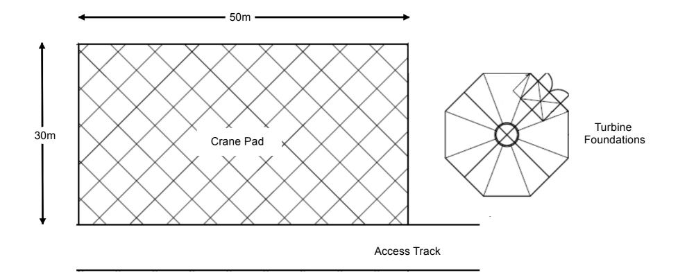
This will comprise crushed stone with a typical thickness of approximately 500 mm, but subject to the specifications required by the selected turbine manufacturer and crane operator, and following detailed ground investigations.
